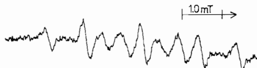
Fig. 1. EPR spectrum of the chloromethyl spin adduct to nitrosodurene recorded 3 min after sonication of dichloromethane solution of 0.1 M [\text{Re}_2(\text{CO})_{10}] and 0.05 M nitrosodurene (sonication time: 3 min).
